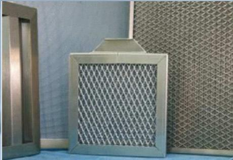
DHD Metal filter cells are made individually to measure. The pressure loss with filter lies between 10 and 70 Pa with a filter depth of 8 – 100 mm. As a frame cutted Platinen are mounted in U form tilted with knitted wire mesh and expanded metal and are welded afterwards with WIG. We are to be covered by our Inhouse manufacturing in the situation of the small series up to the great series everything.
